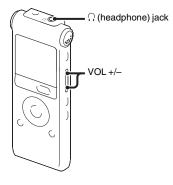
If you connect the supplied stereo headphones to the ∩ (headphone) jack before you start, you can monitor the recording. You can adjust the monitoring volume by pressing VOL +/-, but the recording level is fixed.
